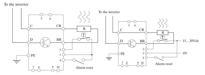
Using the internal power supply of the braking unit
